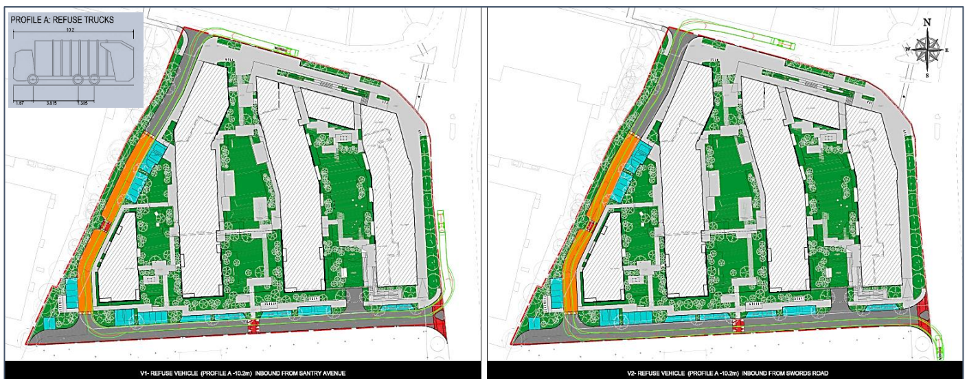
Figure 4-3: Swept Path Analysis for Refuse Vehicle
